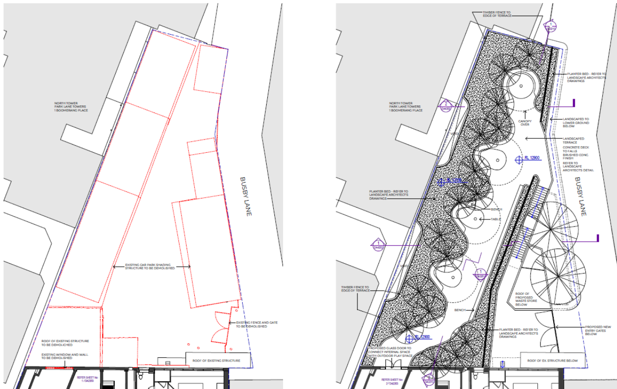
Figure 15: Proposed external ground floor demolition (left) and proposed external ground floor plan of new raised outdoor space (right)
