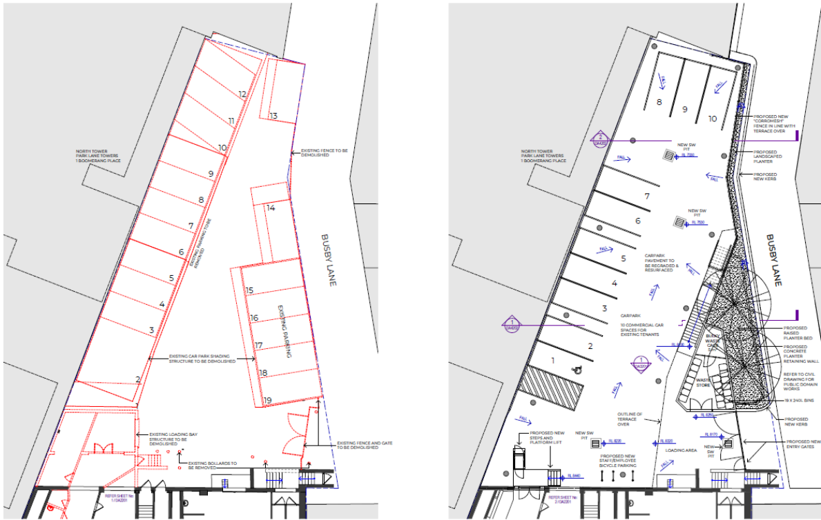
Figure 13: Proposed external lower ground demolition (left) and proposed external lower ground/carpark plan (right)
